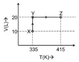
Considering only P-V work is involved, the total change in enthalpy (in Joule) for the transformation of state in the sequence  $X \rightarrow Y \rightarrow Z$  is \_\_\_\_\_.
